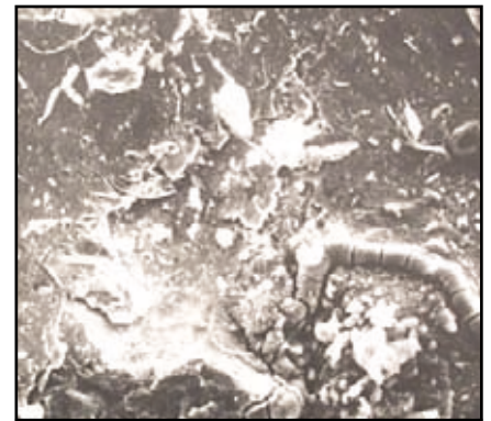
● No HoldTight used: 500x magnification of dry blasted steel plate showing shattered abrasive particles imbedded into the metal profile.
